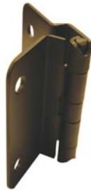
COLUMBIA Offset Hinge: 14 Gauge Type 304 Stainless Steel with a Black Powder Coated finish, allow the door to open 180°.
